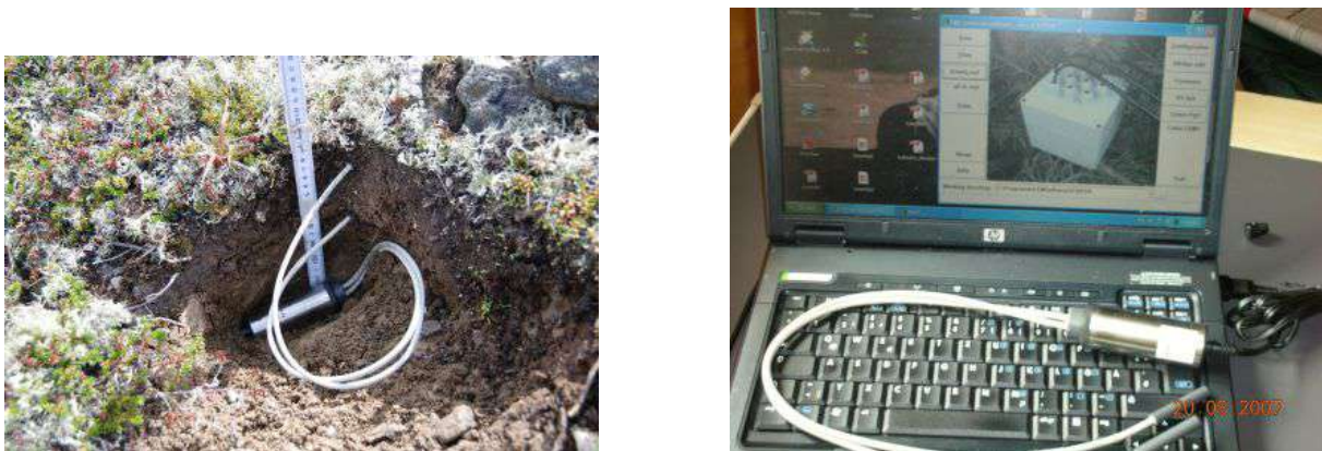
Figure 2.11-D: Soil temperature sensors of the type MINIKIN (left). The sensor itself is a regular Pt100, the head contains an energy source and a storing device. The data are retrieved with the MINIKIN-Software package minikin32.exe (right).
