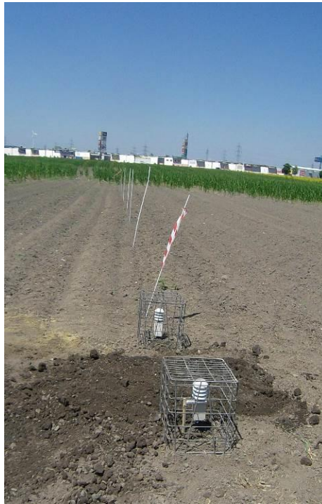
Fig. 12: A line of wireworm bait traps and two data loggers (in the foreground) in a maize field near Bruck/Leitha. The traps were installed in a large area of bare soil caused by severe wireworm damage.
